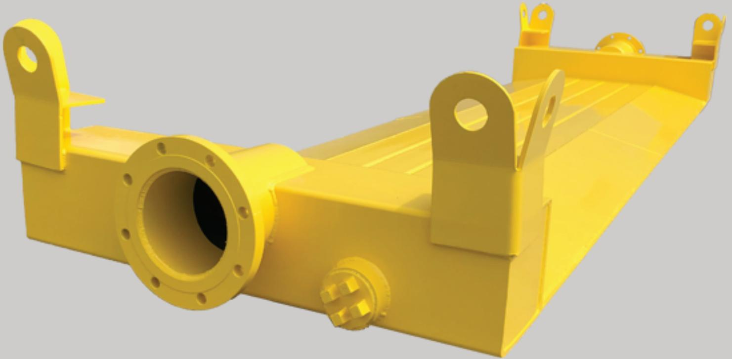
Pinnacle Manufacturing's Road Crossings are designed with job site safety in mind. The low profile design keeps traffic flowing. They are designed for high flow rates with 8 inch and 12 inch flanged connections with 4" cleanout drains. Lifting lugs are built into the stacking corners making transporting and storing easy. All road crossings are SSPC-SP6 blasted and powder coated safety yellow.
